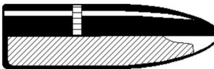
**Open Tip Hollow Point** *The open tip hollow point uses a core shorter than your jacket, and a punch with a probe sticking out to poke a hole in the core.* Like the flat-
