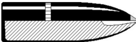
**Lead Tip Hollow Point.** *The lead tip hollow point uses a core that is longer than the jacket, and a punch with a probe sticking out to poke a hole in the core.* The
