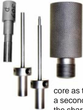
Two special punches are used with the special point forming die. These are provided with and are part of the point forming die, replacing the standard ejection punch. First is the internal punch with a projection to form a cavity in the core as the ogive is formed. This holds the stem of the insert. Then a second punch is used, which has a cavity in the end to fit and hold the sharp end of the insert, and to push it into the bullet nose as the
