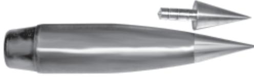
The PF-1-ST or PF-1-HT ULD-TIP point forming/tip seating die is used instead of a conventional point former. Two ejection pins are provided with the special die. The first has a solid end, and is used to pre-shape the ogive and the tip opening size. The amount of core in the jacket is important to allow firm holding of the tip insert stem, and yet not so much that the tip cannot be seated evenly with the jacket edge.
