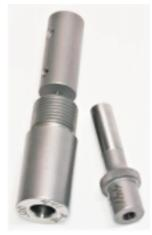
The core seating die is **CS-1-X**, and marked with a "**C**" for Core seat. It's purpose is to seat the lead core into the jacket.
