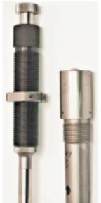
The **FPH-1-X** punch holder has a threaded draw bar. The end of the draw bar screws into the head of the top or external punch. Changing punches is done by turning the knob at the top to unscrew and free the punch. Corbin builds high quality 7/8-14 punch holders with steel split lock rings having wrench flats and hex socket locking screws. The punch holders are black oxide finished. Complete FPH-1-X, \$149.
