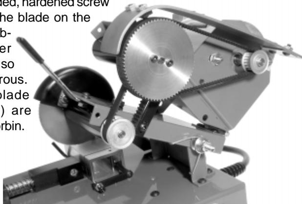
The SAW-2 should NOT be disassembled when replacing belts. The angle between plates is carefully adjusted to compensate for belt torque, to keep the belts running straight without rubbing on the pulley. If you see a build-up of rubber on the side of the reducer pulley on the upper spindle, it means the saw is not properly aligned and belt life may be shortened.
