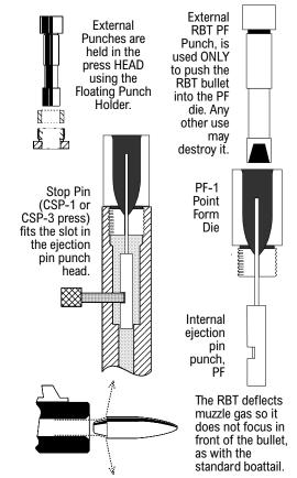
Never try to swage a component that will not go into the die by hand. The swaging operation depends on each component being slightly smaller than the die bore, and increases the bullet diameter a little with every step.
