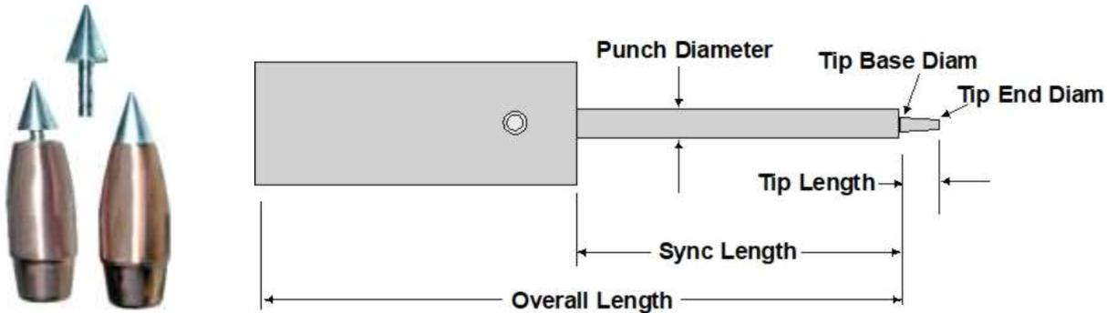
First the ogive is formed on the bullet and the centered hole is created by the T1 punch in the lead core to grip the stem of the tip insert. Then the internal punch is changed to a second ejector, designated as T2, which has a cavity in the end, designed to eject the bullet from PF-1-HT die while maintaining the perfect alignment and centering of the insert.
