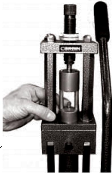
Putting the lead cylinder in the ball swage die
