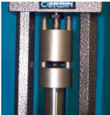
Forming the ball as the two halves of the die slide together on the guide rods
