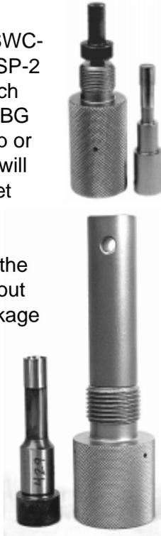
The LSWC die screws directly into the ram of the Corbin press. The internal punch slides up and down inside the die, and ejects the bullet on the down stroke. A stop pin (in the CSP-1 press) or a knock-out bar (in the larger Corbin presses) comes to rest against the end of the internal punch and stops it on the down stroke, while the ram and die continue down. This pushes the bullet out.
