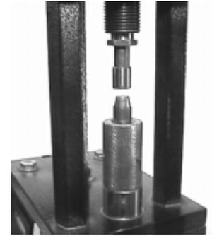
If the die does not appear to move far enough, or the handle stops before it has made a complete 180-degree arc, you probably have the press in the reloading or long-stroke position with the stop pin in place. This may bend or shear the stop pin if you press hard enough. Always put the press in the short stroke, or swaging, mode by moving the ram link pin to the set of toggle holes that give the shorter ram movement. Instructions and pictures are found in the papers that come with your press.
