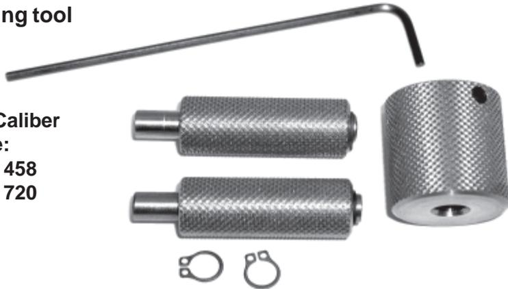
This is a special set of hardened tool steel rollers with hardened axel pins, used to replace the standard rollers and pins on the HCT-2 lead bullet knurling tool, to allow use on jacketed bullets. One purpose is to expand the diameter of a jacketed bullet slightly. Another is to provide a grip surface on the otherwise smooth bullet for use in certain kinds of sabot rounds.
