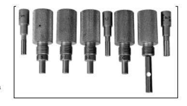
internal punch for the CS-1, and a POINT FORM (PF-1) die with both RBT and FB external punches.
