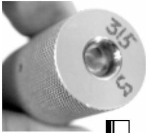
The CORE SWAGE (CSW-1) screws directly into the press ram, and adjusts the lead core weight. It has bleed holes around the circumference.
