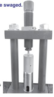
To check alignment, you can leave out the swaged material and lower the punch into the die about half its distance, then secure the punch retainer bushing by hand. The lock ring can be secured for this test but will be adjusted for the actual swaging operations.
