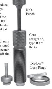
peat this until the core weighs what you want. Then lock down the die and process all the other cores you have cast or cut slightly heavier (from 3-10 grains more) than the desired final weight. Core weight plus jacket weight is bullet weight: for a 55 grain bullet, set the scale at 55 grains, put the jacket into the scale pan, and then adjust the core weight until the scale balances.
