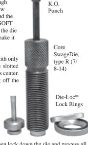
peat this until the core weighs what you want. Then lock down the die and process all the other cores you have cast or cut slightly heavier (from 3-10 grains more) than the desired final weight. Core weight plus jacket weight is bullet weight: for a 55 grain bullet, set the scale at 55 grains, put the jacket into the scale pan, and then adjust the core weight until the scale balances.
