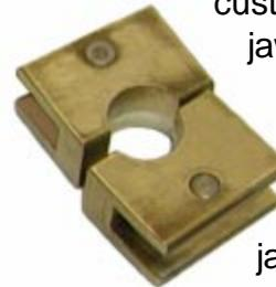
BLANK JAWS are also available to make your own puller. The hole should be drilled and reamed just slightly larger than the bullet to be pulled, but with the jaws clamped together on a shim of about .015-.020 inches thickness. This creates a crush fit oval hole without corner pinching.
