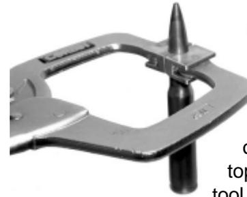
(If available, use a 7/8-14 adapter in the press top to reduce the size of the hole and allow more support for the tool. A large steel washer with 9/16 hole can also be placed over the threaded hole in the press top, to provide a level support for the tool.)
