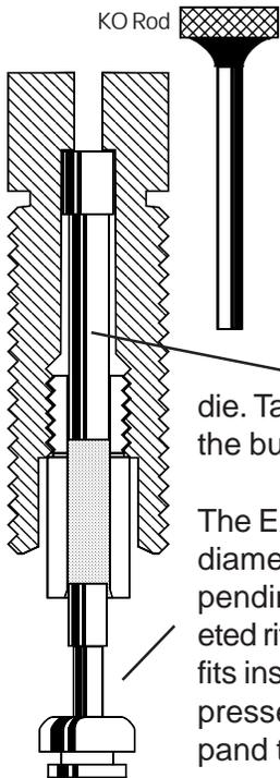
The first die is the CORE SEATER. It is used to expand the jacket to proper diameter while pressing (seating) the lead filling (core) into the jacket.
