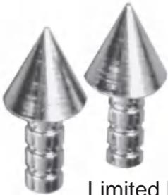
The new tips are different from Corbin's well-known ULD-TIP inserts (Ultra Low Drag). Pin-Points have a 25-degree nose cone, with a 0.1-inch diameter grooved stem, so they allow the swaging of a shorter ogive in the same weight, or a heavier weight in the same length.
