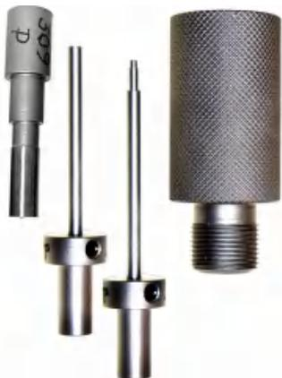
All it takes to add this bullet to your product line is a single die (PF-1-ST for the S-Press, or the PF-1-HT for the CSP-2 Mega Mite or CHP-1 Hydro Press). This is the same basic design as the well-proven ULD-TIP seating point form die, but with proper angle and ogive to match any caliber from .358 to .510 diameter. When ordering, just check the "Pin-Point" option rather than the "ULD-TIP" option.
