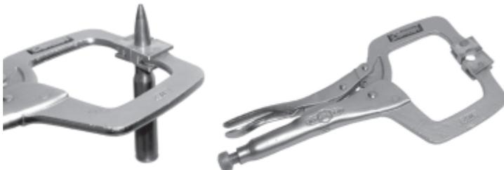
Lowering the handle then pulls the bullet cleanly, safely, without the shock of an inertial hammer puller.
