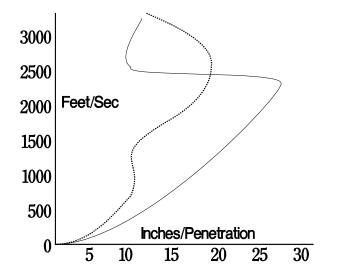
Penetration versus velocity: two bullets, one expanding (dotted) and the other solid, fired to destructive impact.
