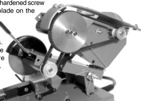
The SAW-2 should NOT be disassembled when replacing belts. The angle between plates is carefully adjusted to compensate for belt torque, to keep the belts running straight without rubbing on the pulley. If you see a build-up of rubber on the side of the reducer puller on the upper spindle, it means the saw is not properly aligned and belt life may be shortened.
