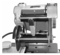
back legs of the saw are longer than the front legs, so that the saw sits at an angle to allow cut pieces to roll forward. The motor and arbors are set at a slight cant to compensate for belt torgue. Do not "straighten out" the relation of the upper and lower mounting plates, as this will cause excess belt wear and breakage.
