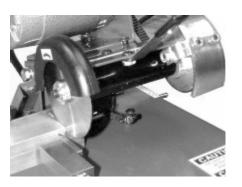
When cutting long pieces of tubing in the SAW-2, it is advisable to support both ends of the tub-
