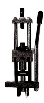
press whatever. All parts are machined steel, with a "grenade-pin" to quickly release the ram linkage and reposition it for the desired stroke length.
