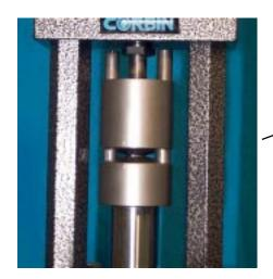
Forming the ball as the two halves of the die slide together on the guide rods
