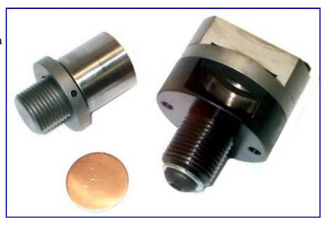
The strip is pulled through the slot, the handle moved up and down in short strokes, just enough to cut the metal, and the strip advanced to the next position by observing the relation of the last hole in the strip compared to the edge of the die, leaving enough metal between holes for a good disk to be cut on the next stroke.
