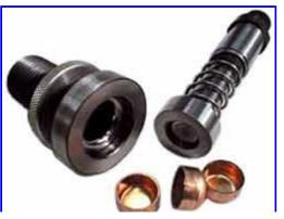
the top of the die, and the cycle is repeated. The die forms a short, thick-walled cup of about .600 diameter.
