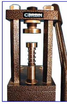
The .600 diameter cup is then lubricated and placed over the .500 first draw punch, which screws directly into the ram. The .500 draw die screws into the top of the press, and the press is set for the long stroke or reloading mode. The .600 diameter cups are drawn to .500 diameter, while the walls are made thinner and the length increases.
