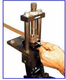
After the disks are cut, the cupping die and punch assembly are put into the press. The cupping die itself goes into the ram from the bottom side, which is the opposite of most dies. The spring-supported guide and punch screw into the ram. A lubricated disk is placed in the top of the guide, which in turn is held in position on top of the punch.
