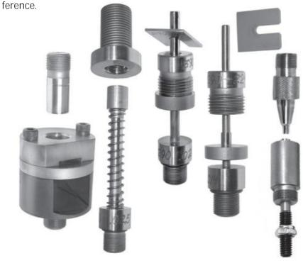
The JMK-1-S is designed to operate in the CSP-1 S-press. It is not suitable for a reloading press. The jacket length, diameter and wall thickness are limited by the stroke of the S-press. Longer, larger, or thicker walled jackets may be made with the CHP-1 Hydro Press using the JMK-1-H manual feed, or JMK-2-H auto-blank/cup jacket makers. The kit consists of a blanking die (left), a cupping die, one or more drawing dies with guides and stripper plates, and a trim die to adjust the final length.
