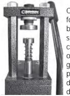
Continue to raise the ram so that the disk is formed into a cup. Do not "coil-bind" the spring by raising the ram higher than necessary, or the spring will be ruined. If the disk is turned into a cup and passes freely into the threaded portion of the die, so it is loose in the die, then you have gone as far as needed. The next cups will lift the previous ones out the top of the die. Use CDL-2 draw lube on the disk (both sides) to preserve die life and reduce friction.
