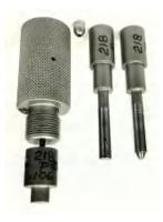
If you get flashing or ragged thin lead extrusions at the BASE of the slug, it is almost certainly either a damaged punch that was driven into the ogive of the die at least once, OR the punch was fitted to another die, has been dropped on a hard surface and "dinged" the edge, or has been in some other way damaged at the edge.
