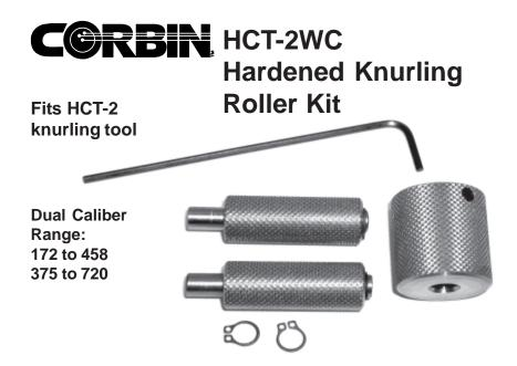
This is a special set of hardened tool steel rollers with hardened axel pins, used to replace the standard rollers and pins on the HCT-2 lead bullet knurling tool, to allow use on jacketed bullets. One purpose is to expand the diameter of a jacketed bullet slightly. Another is to provide a grip surface on the otherwise smooth bullet for use in certain kinds of saboted rounds.
