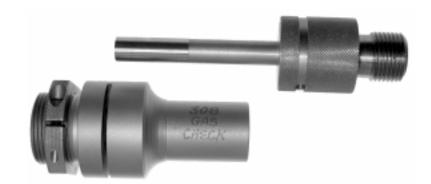
This die and punch set is used in the Corbin CSP-2 and CHP-1 presses to punch a stirp of copper tubing, normally 1-in wide by .030-in thick, into proper diameter disks which are then used to make gas checks.
