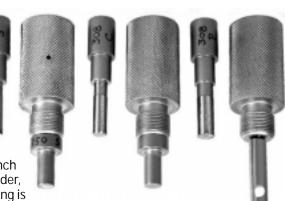
removed from the bottom of the punch holder and is placed over the external punch, and then screwed back into the bottom of the punch holder to secure the punch. The punch holder screws into the press head, so the punch faces the ram. (Large diameter punches have their own captive threaded bushing: do not remove this from the punch.)
