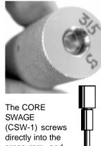
(CSW-1) screws directly into the press ram, and adjusts the lead core weight. It has bleed holes around the circumference.
