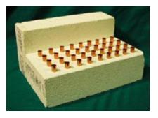
even a standard wood bit. A pattern of 32 holes per brick can be made using the template that comes with the Corbin BL-KIT (two heat treatment blocks). One block should be drilled, and the other can be used as a backstop for the flames, to reflect the heat back on the reverse side of the jackets.
