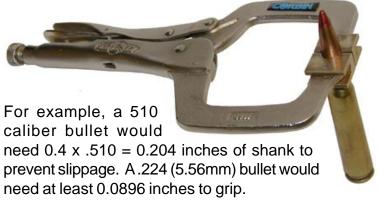
Bullets seated too far into the cartridge case to have enough parallel shank exposed must be pulled with an intertial tool, or by an edged grip which dig into the curved section of the bullet that is exposed above the cartridge case neck.
