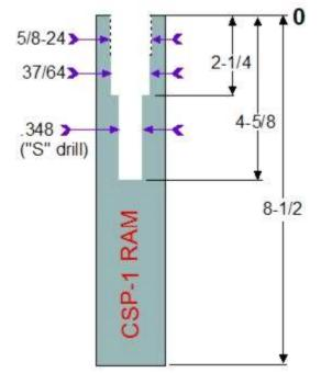
The .348 diameter hole in the drawing can fill partly with debris from reloading and swaging operations, so that the end of the internal punch hits the compacted material. This in turn puts the entire force of press against the punch head, which in the point form die is pinned to the frame through the stop pin. All of the force of the press is now applied to the stop pin, breaking it.
