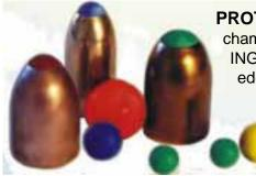
PROTECT THE TIP of your bullet from deforming in the magazine, during chambering, or in flight by using a small size poly ball at the tip. INSURE FEED-ING in auto-loaders by using a larger poly ball at the tip, trapped by the jacket edge (just past the mid-point on the diameter). The ball tip can even be set to turn, like a ball bearing!
