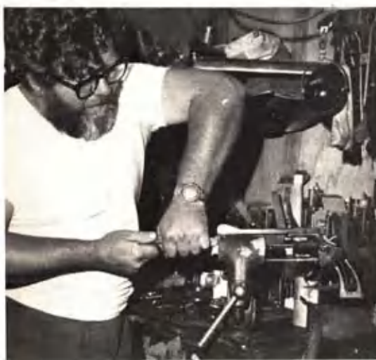
Left: Bob Day cuts forcing cone in new barrel being installed on customer's Smith & Wesson M-10.
