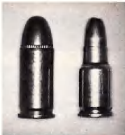
Left: An original .32ACP round and the same case wildcatted to Flea with the 37 gr. bullet.
