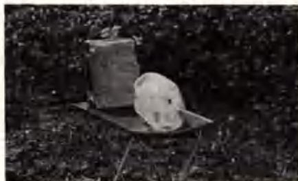
Water-filled jug is shattered, but paper background shows no signs of pellet penetration.
