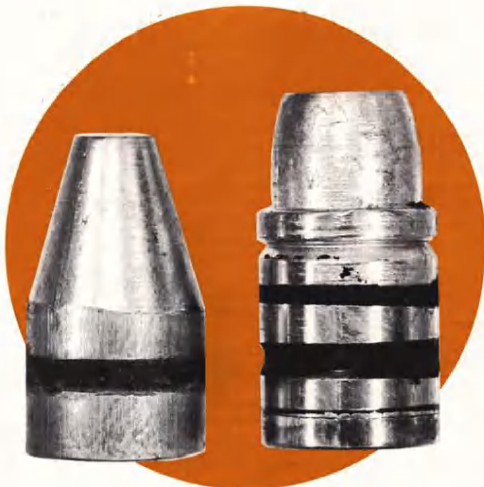
Typical cast lead lubricated bullets. Bullet on right based with gas check, bullet on left has been improperly resized.
