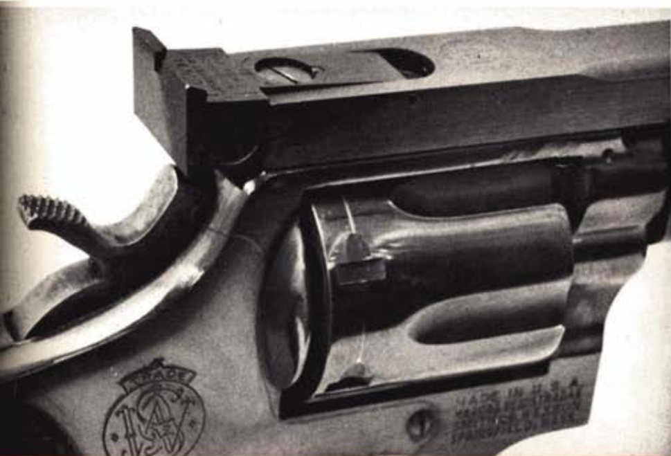
The rear sight is of Day's own design and affords a wide, black, square sight picture. Extra long elevation screw allows for full adjustment.
