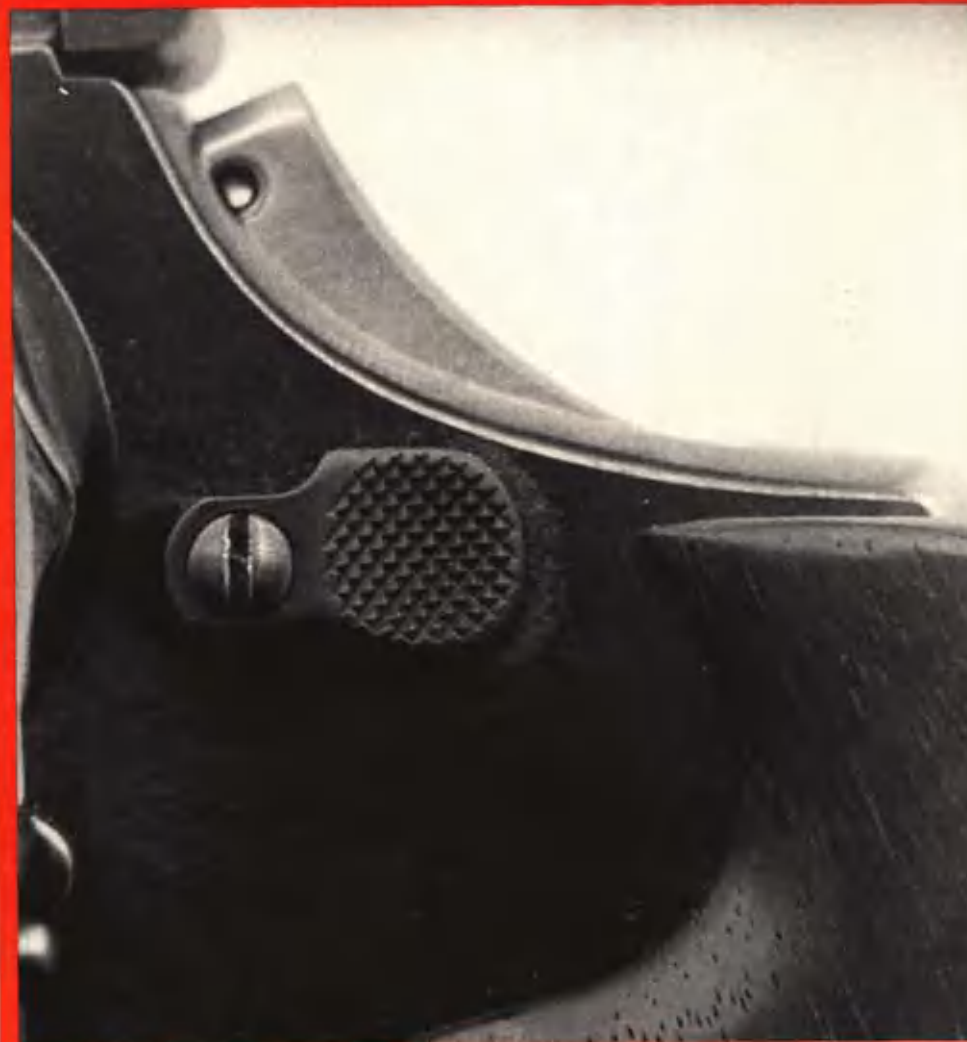
Close-up shows two desirable Combat modifications. Hammer has been bobbed for D.A. only shooting and cylinder latch has rounded edges to prevent cut thumbs after hot load recoil. Both are simple jobs.
