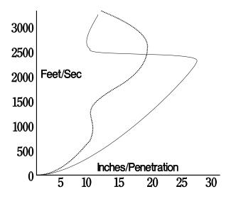
Penetration versus velocity: two bullets, one expanding (dotted) and the other solid, fired to destructive impact.
