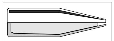
The SPIRE POINT bullet would be called a conical in shorter, pistol styles. It uses a straight, angled nose rather than a curved ogive nose, joining the shank at an angle.
