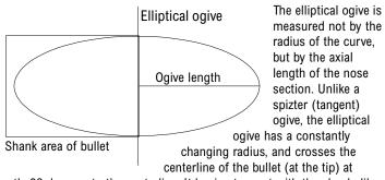
exactly 90 degrees to the centerline. It begins tangent with the shank, like a spitzer ogive. The two most practical lengths are the 3/4-E and the 1-E ogive, for pistol and rifle respectively.
