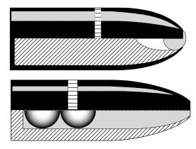
Bullet Balls Plastic spheres can be used either in the tip of a hollow point bullet, as a kind of pneumatic expander, or to shift the balance and lighten the bullet, for high speed yet stable projectiles.
